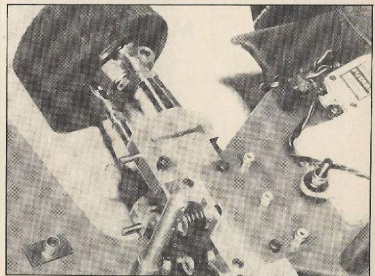
Very neat bellcrank arrangement to enable a Preston sleeve carb to be used on his OPS in John Hale's o.d. "After" Rapier design and still enjoy a straight push/pull for brakes and throttle.
