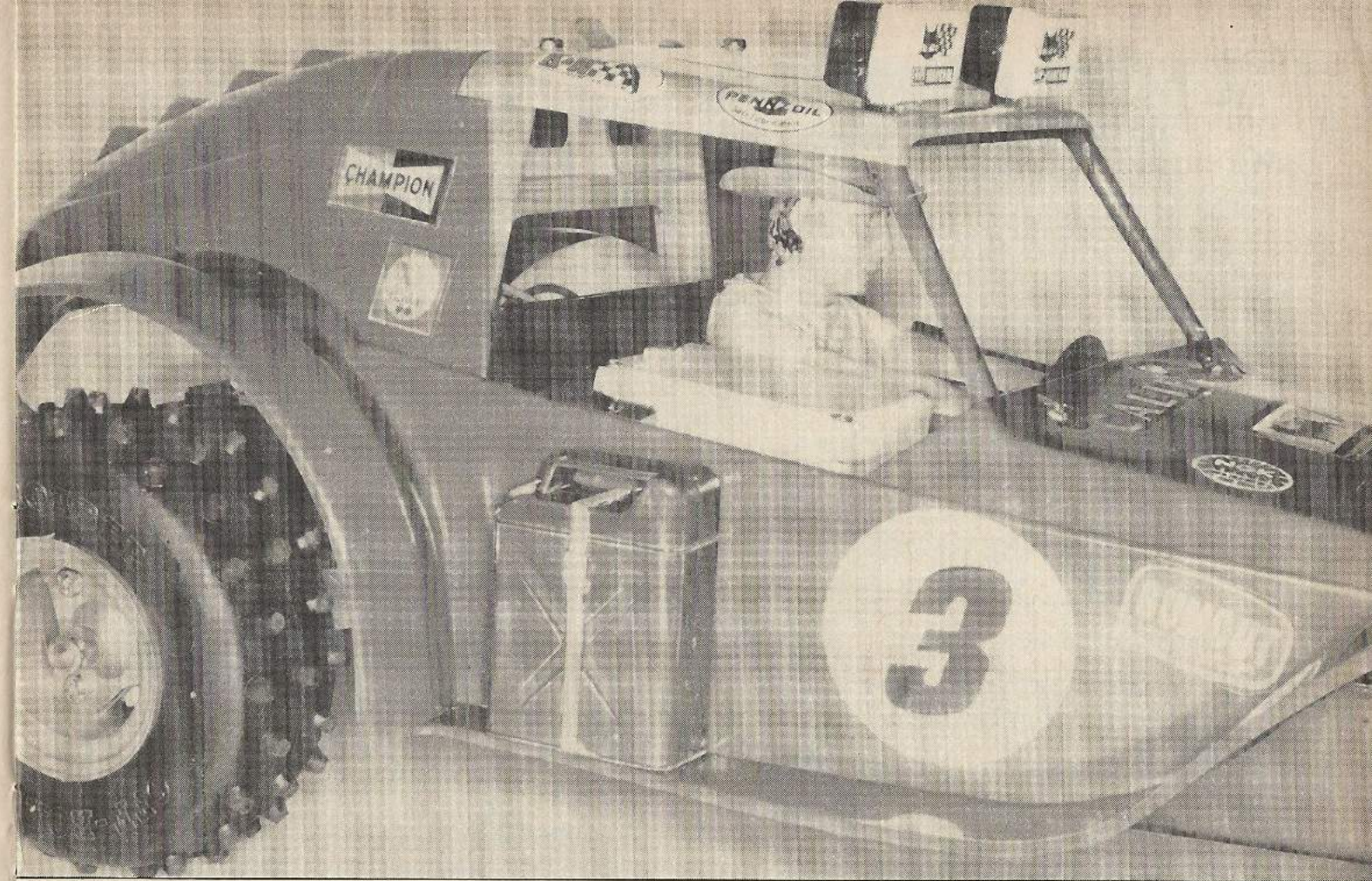
Shows how spare place by driver has been cut out to take Rx, with its conveniently located crystal for quick change. On/off switch is behind the rx.
